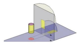
The two views dihedral (in plan and elevation) would in this way. After the rotation of the object dihedral projections are always correlated.
