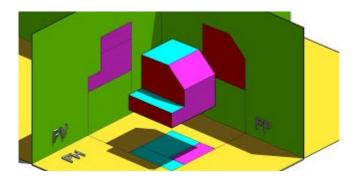
In the figure we see in yellow what is projected in the vertical plane, in red and green on the green horizontal and the plane of the profile.
