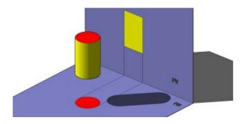
Then turn the vertical plane 90 degrees until it coincides with the horizontal axis of rotation taking as the ground line. The rotationcauses the two views are perfectly aligned in lines orthogonal to the ground line.
